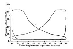
FIG. 38. Steam engine indicator card on displacement base.
